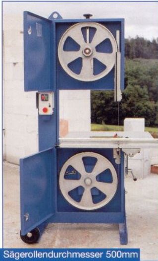
Sägerollendurchmesser 500mm Saw wheel diameter 500mm
